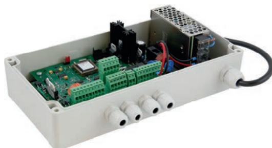
Control unit, incl. power pack, in plastic housing
